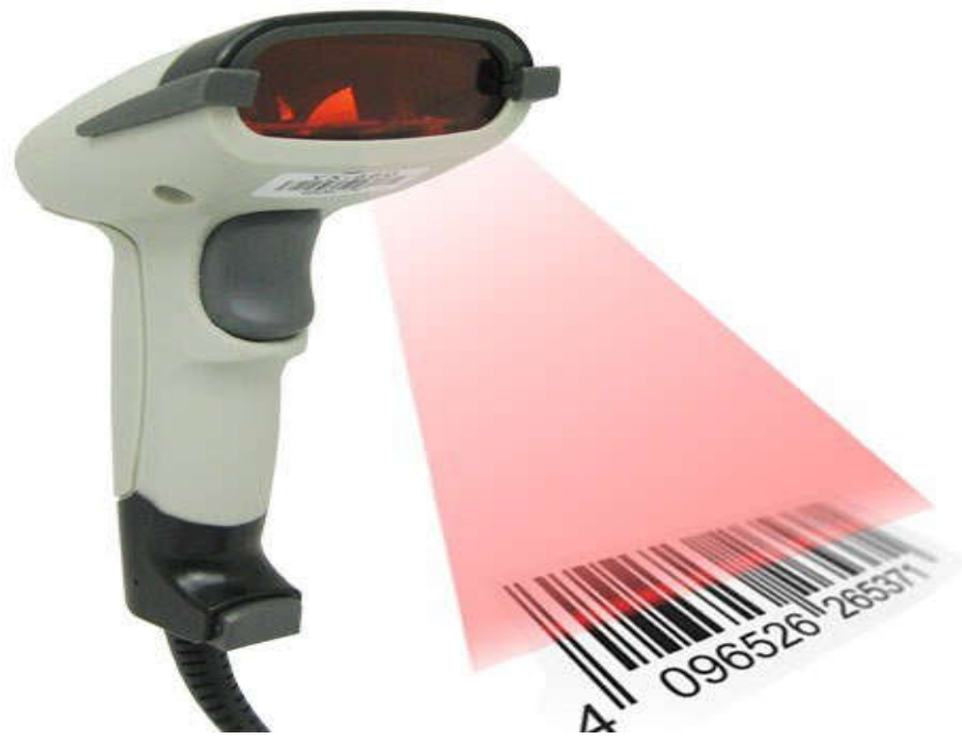
Figure.1. Barcode system: scanning device (reader) and the barcode card.
