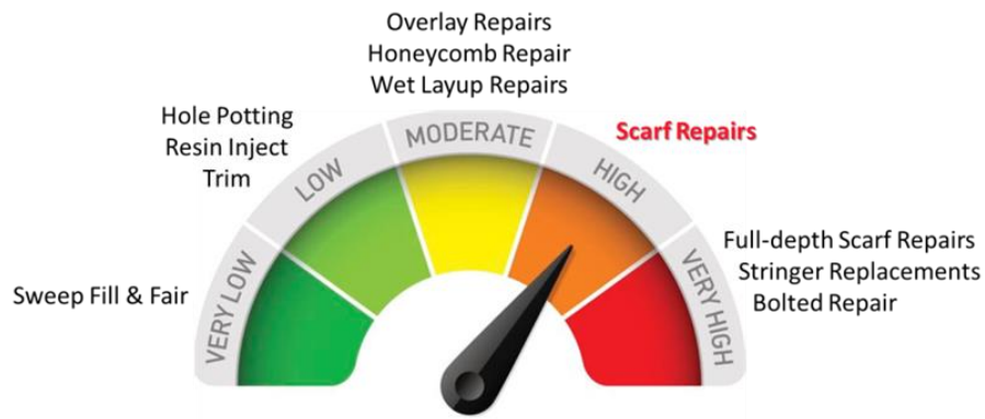
Figure 3.2: Repair types and repetitiveness table.
