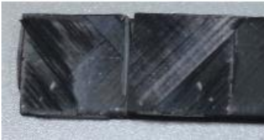
Figure 4.18: Breaking away part in the bonded area.
