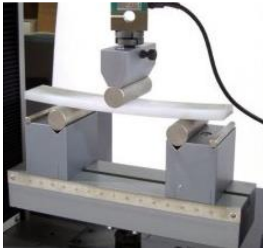
Figure 3.14: The three point bending test set-up. Taken from [50].
