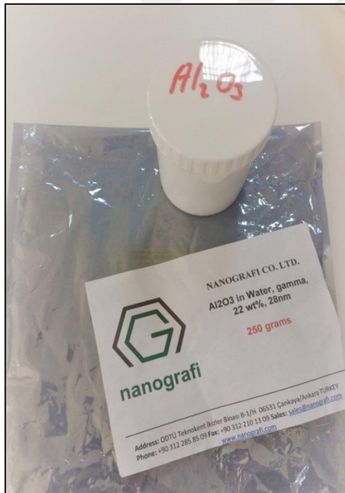
Figure (3.12): The \text{Al}_2\text{O}_3 /water and \text{TiO}_2 /water nanofluids supplied by Nanografi Company (Turkey).
