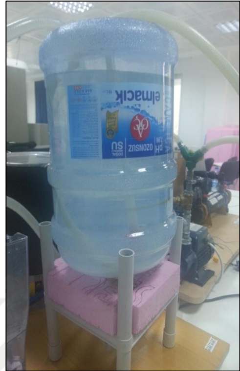
Figure (3.8): The cold fluid tank.
