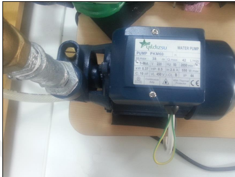
Figure (3.6): The cold fluid pump.
