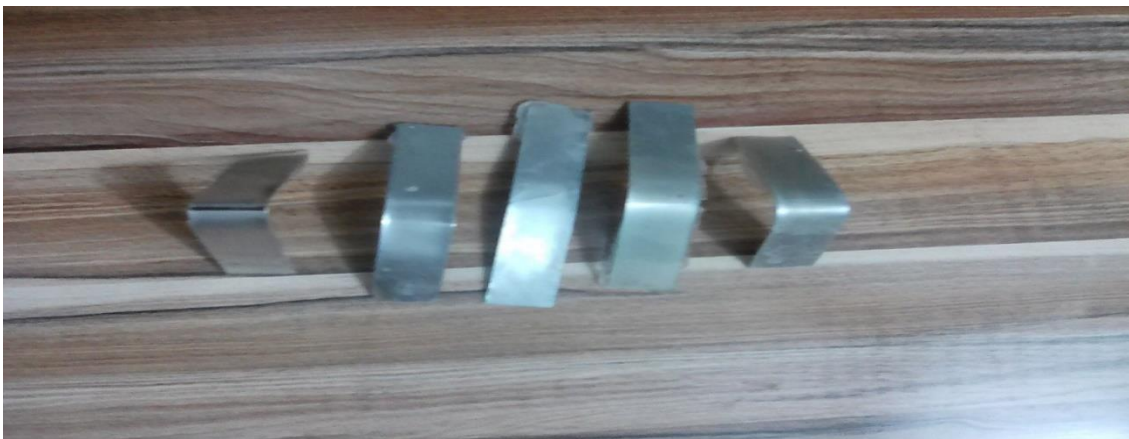
Figure 3. 19: Specimens after bending
