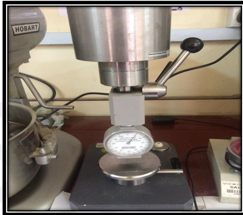
Fig (3-14) Hardness Testing Equipment (Gewicht Shore D ) serial No.3279 and manufacture company Elcometer, in Material Engineering Department, University of Technology-Baghdad-Iraq.
