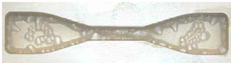
Figure 3-7 Air bubbles in manufactured samples
