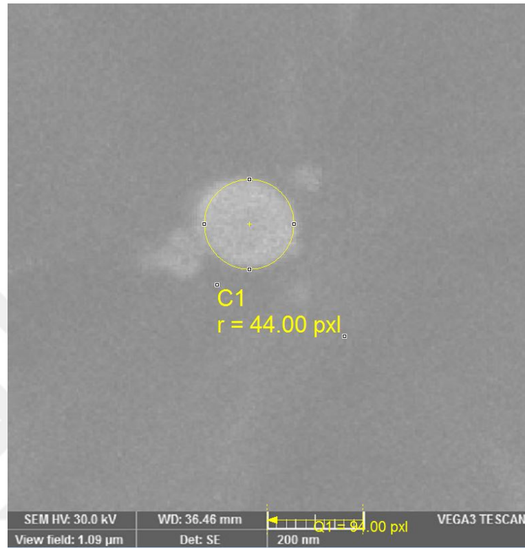
Figure 4-16 SEM image with measuring tools applied to the PMMA – Al 2 O 3 tensile test specimen at a fracture
