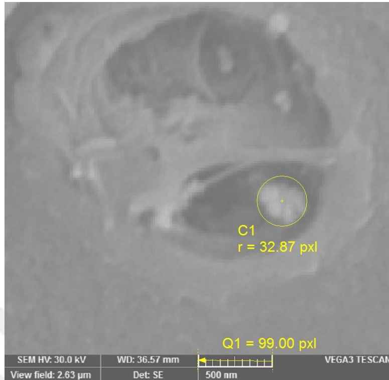
Figure 4-19 SEM image with measuring tools applied to the PS - Fe_3O_4 tensile test specimen at a fracture
