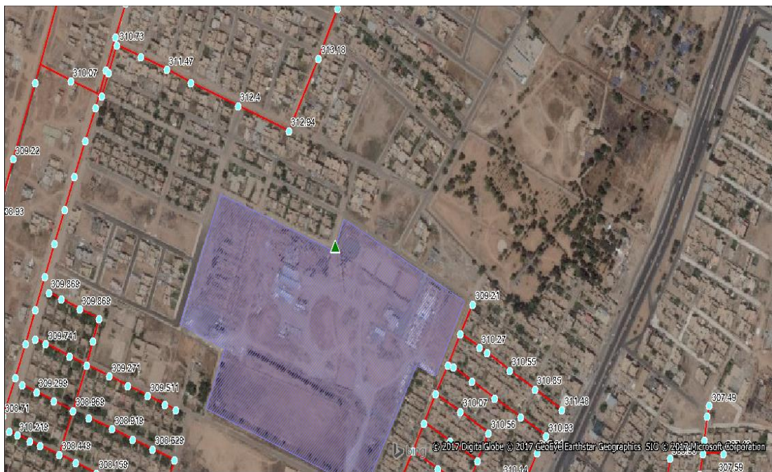
Figure 5.2 Suitable manholes from A1MH2
