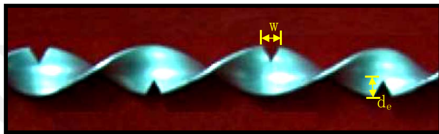
Figure 1. 6 : Dimensions of V-cut twisted tape
