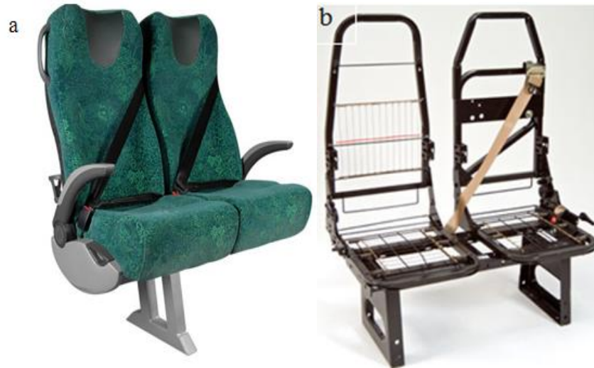
Figure 4.3. a) A complete bus seat (Anonymous,2016d) b) A bus seat frame (Anonymous,2016e)
