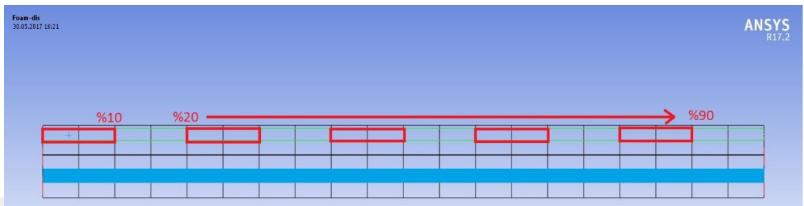
Figure 49: Patch division lengths and increment direction for front MFC Patch
