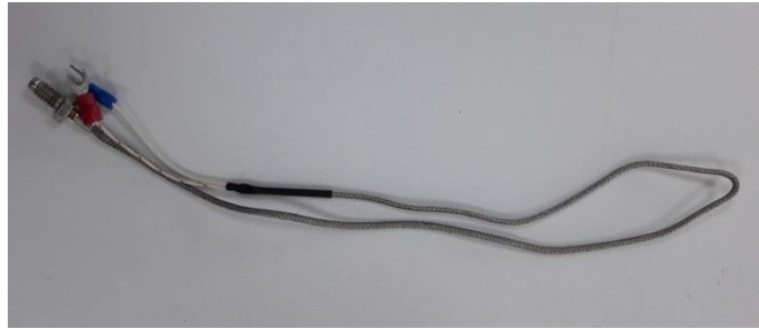
Figure 3. 11: Thermocouples type (K 0.2mm)
