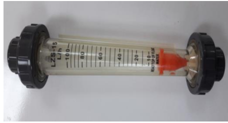
Figure 3. 9: Water flow meter.
