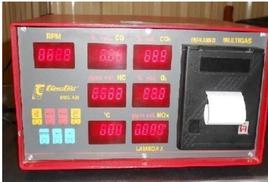
Figure 3.9 Exhaust gas Analyzer
