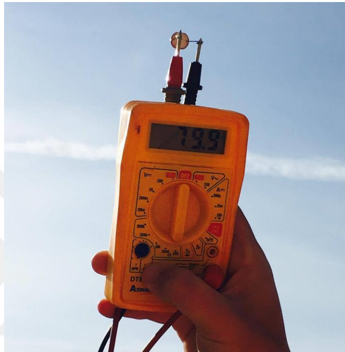
Figure 3.23: Measuring the LDR resistance.
