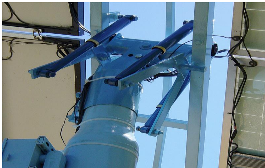
Figure 2.3: The passive tracker.
