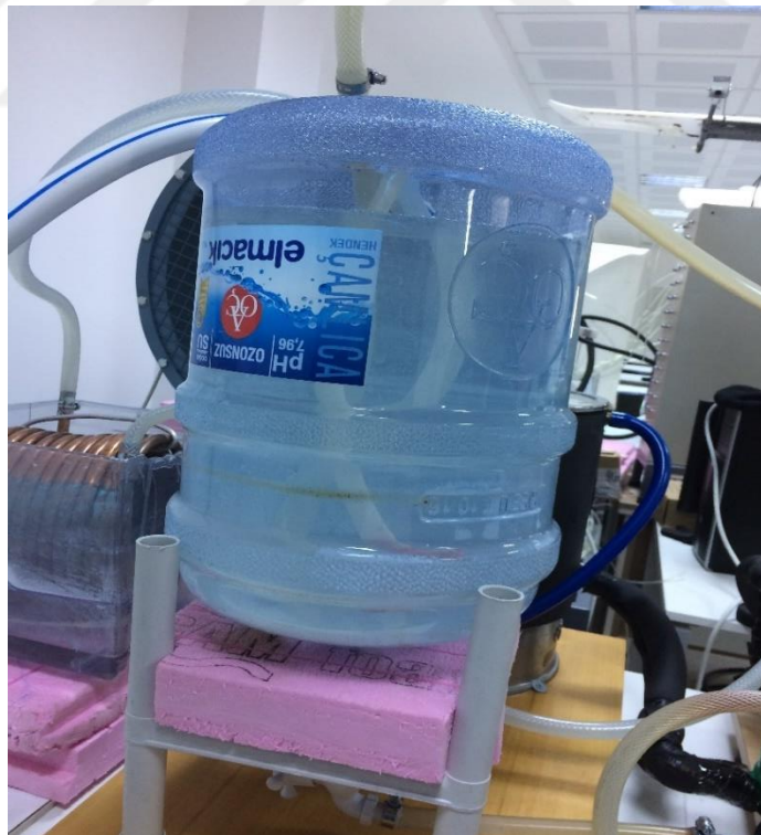
Figure 3.9: The cold fluid tank
