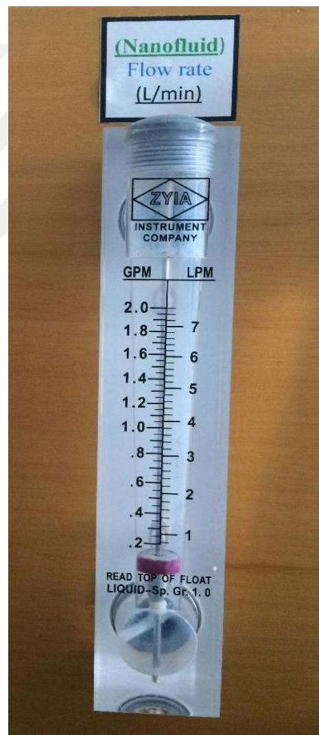
Figure 3.12: The flowmeter for a cold loop.
