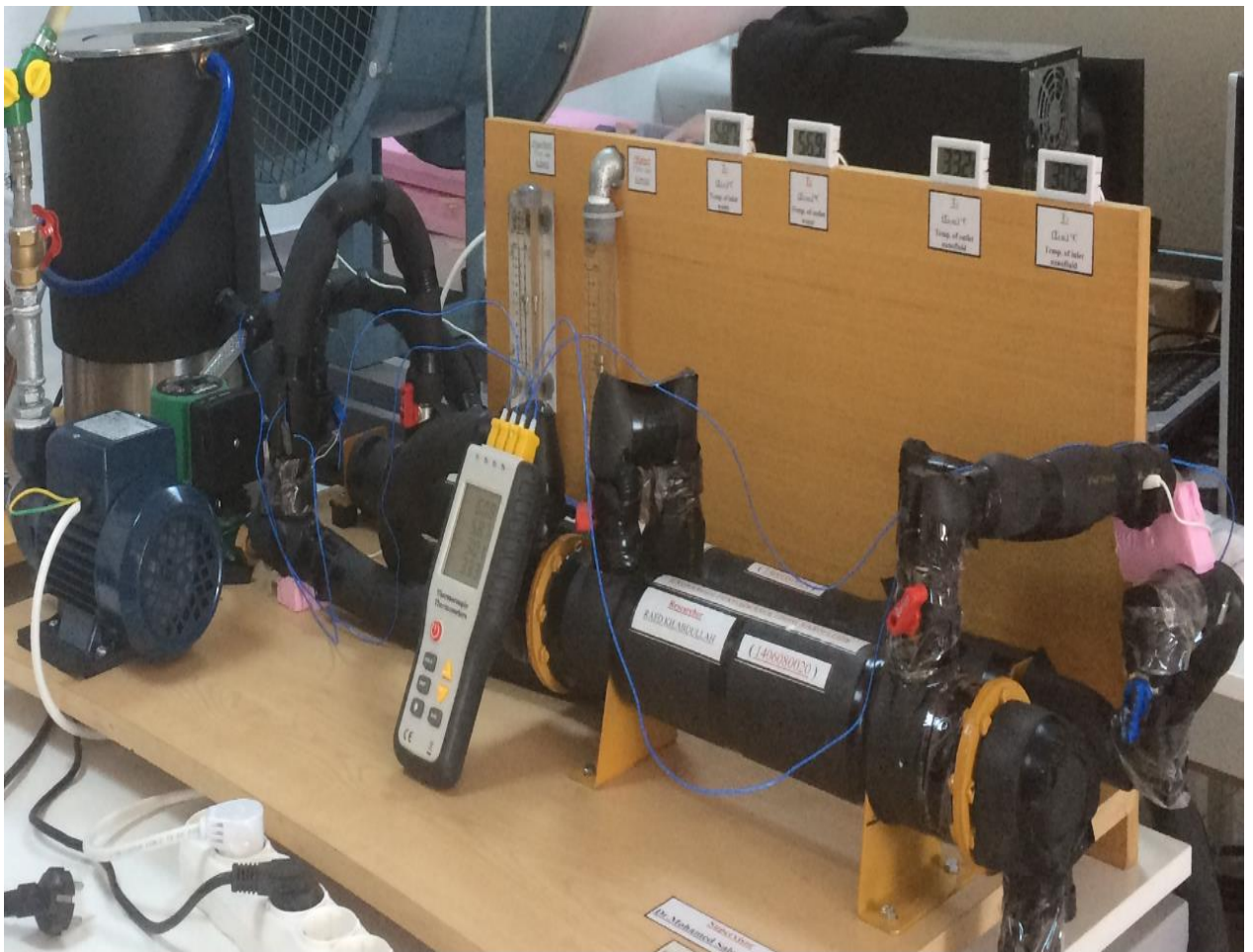
Figure 3.5: The insulation of the double pipe heat exchanger, storage tanks, and the inlet and outlet pipes connected to the double pipe heat exchanger.
