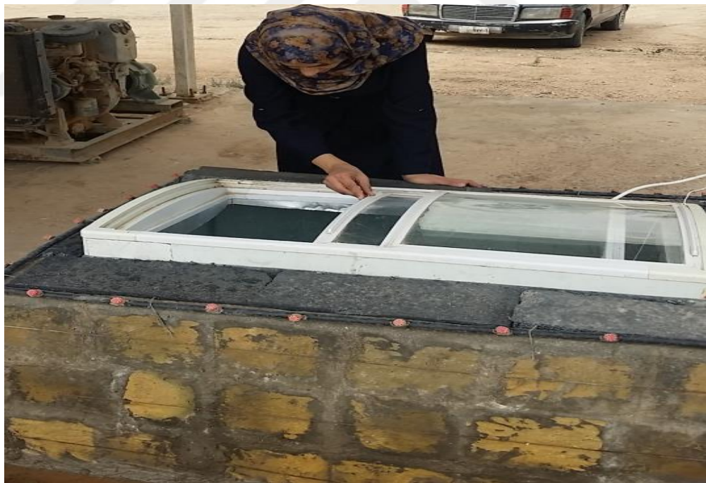
Figure 3.4: Installing the Metal Basin inside the External Basin and Fill the Interval Distance by Water
