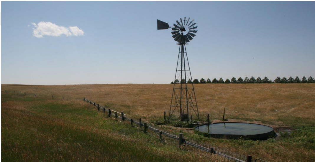
Fig. 1.2 A windmill for water pumping with steel-bladed [4]
