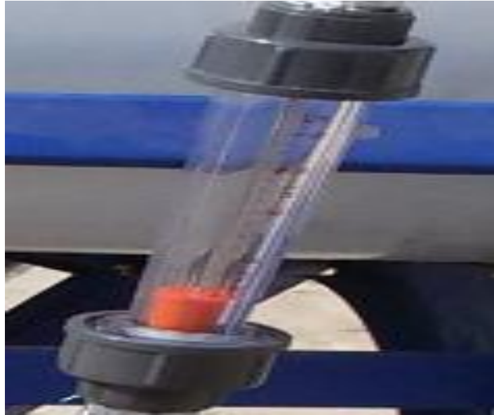
Figure 3.7 Water Flow meter
