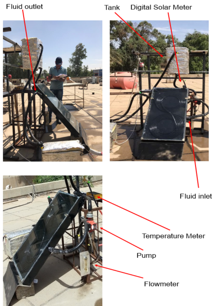
Figure 3.2: Experimental set-up of FPSC
