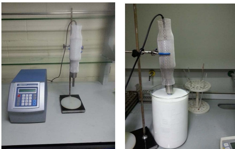
Figure 3.12: (a) The Ultra-sonicator and (b) mixing of the nano-fluids
