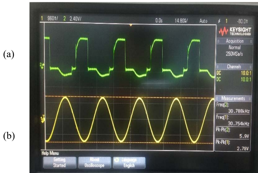
Figure 3.14: Signals from the transmitter and receiver coils (a) The transmitted signal, and (b) The received signal
