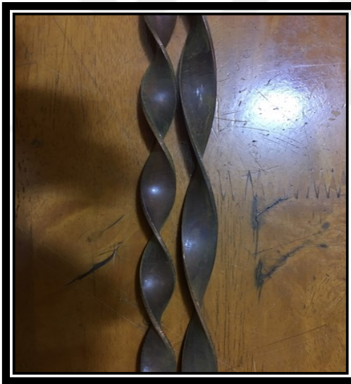
Figure 3.6: Photograph for Typical twisted tape types with different twist ratio.
