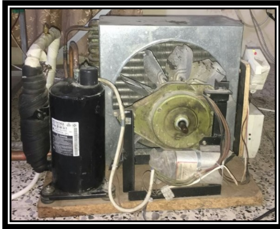
(a) Fan and Compressor
