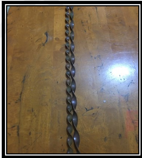
Figure 3.6: Photograph for Typical twisted tape types with different twist ratio.
