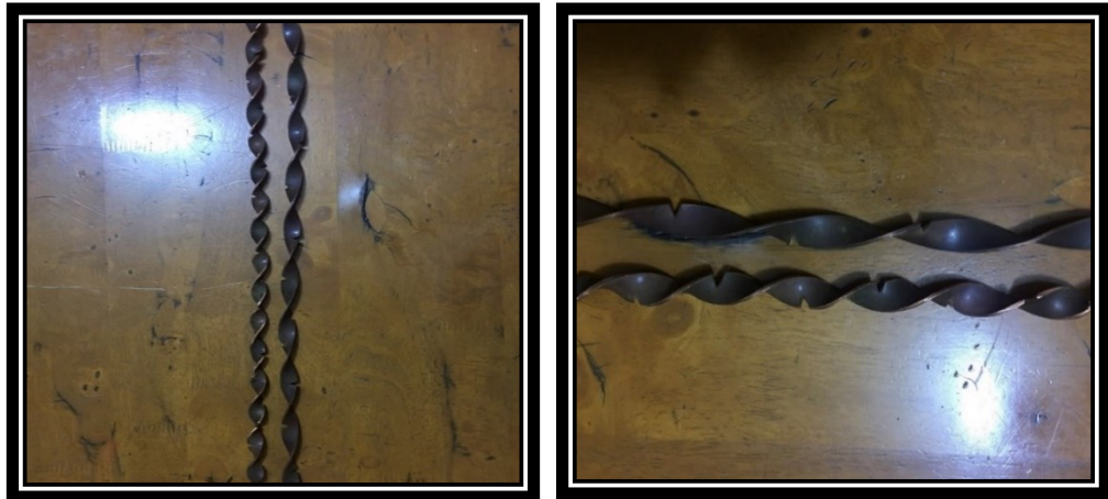
Figure 3.7: Photograph for V-cut twisted tape types with different twist ratio.
