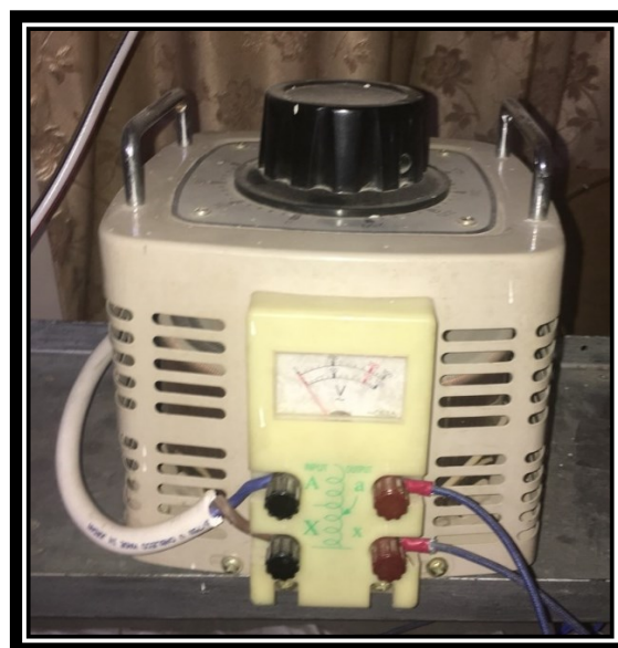
Figure 3.4: Variac voltage transformer.
