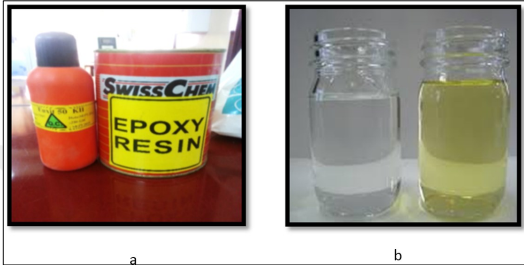
Figure 3.2: (a) The cans of epoxy resin (EUXIT 50 KI) and hardener, (b) The sample of epoxy resin and hardener.
