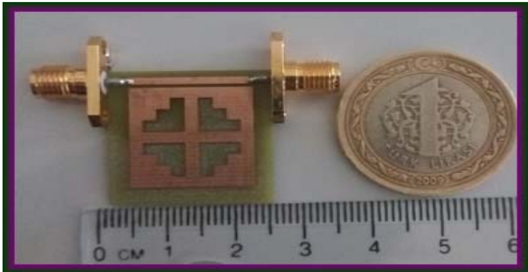
Figure 37: Photograph of the fabricated quasi fractal BSF using FR4 substrate.
