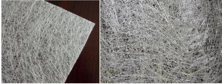
Figure 2.11: Chopped-strand mat contains randomly distributed fibers.
