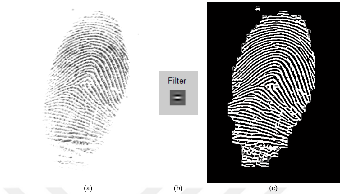
Figure 3.27: Localized image filtering results (a) The original low-quality fingerprint, (b) Gabor Filter, (c) Image enhancement.
