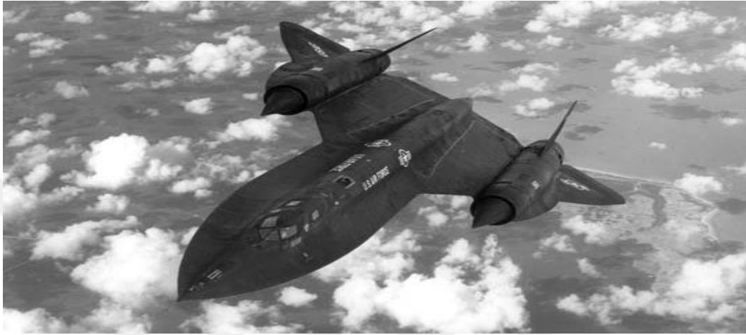
Figure 4: SR71 aircraft: first use of beta alloys in aerospace structures [7]
