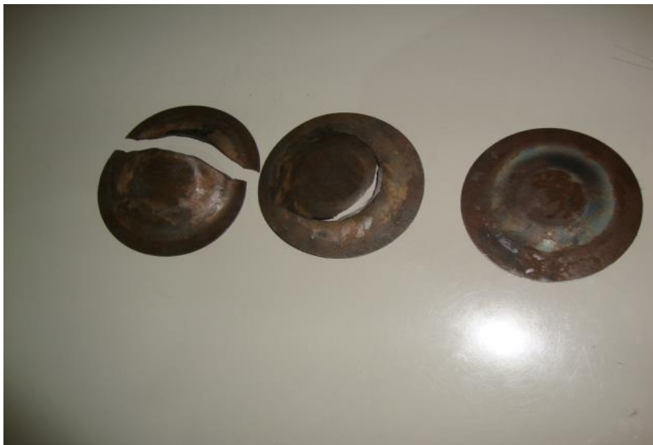
Figure 60: Ti-6Al-4V alloy blank after forming with fracture in second experimental.
