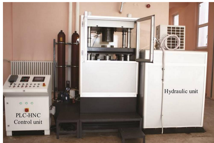
Figure 26: Showing hydraulic press system used in experimental work [28].
