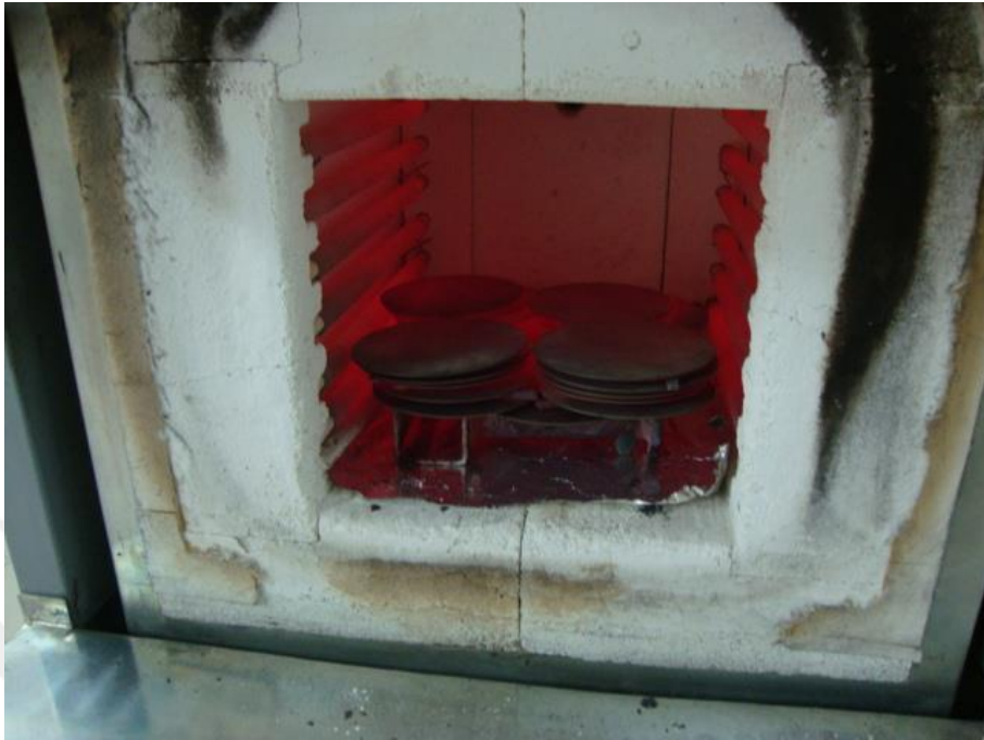
Figure 40: Blanks after finished heat treatment.
