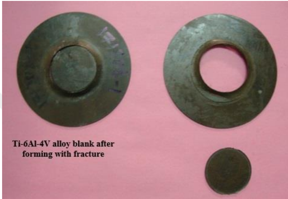
Figure 59: Ti-6Al-4V alloy blank after forming with fracture.
