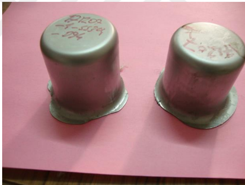
Figure 67 : Stainless Steel type (304) cups forming in same forming tools for (Ti-6Al-4V) sheet alloy.
