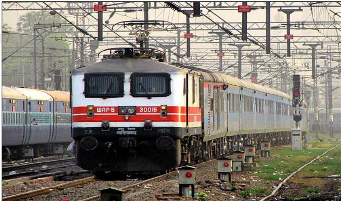
Figure 3.13: Electrical train with catenary line [31].
