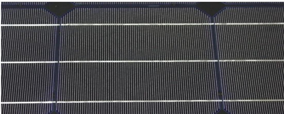
Figure 3.1: Monocrystalline solar cell (3 Bus) [13].
