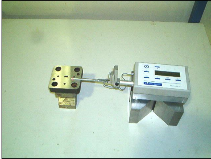
Figure 3.9: Surtronic 3+ device to measure the surface roughness
