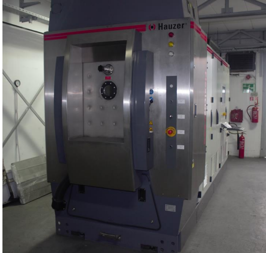
Figure 3.11: Hauzer Rapid-Coating-System (HCS) deposition machine
