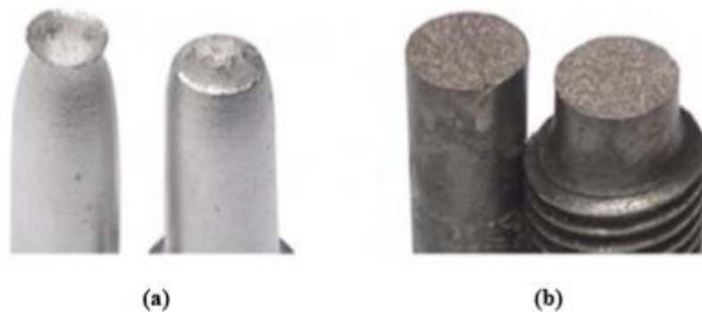
Figure 2.26: (a) "Cup and cone" fracture formation observed in aluminum. (b) A brittle fracture found in not-so-tough steel.
