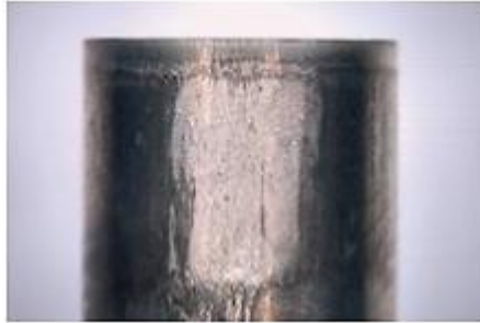
Figure 2.13: Galling on punch face [Uddeholm and SSAB 2008]
