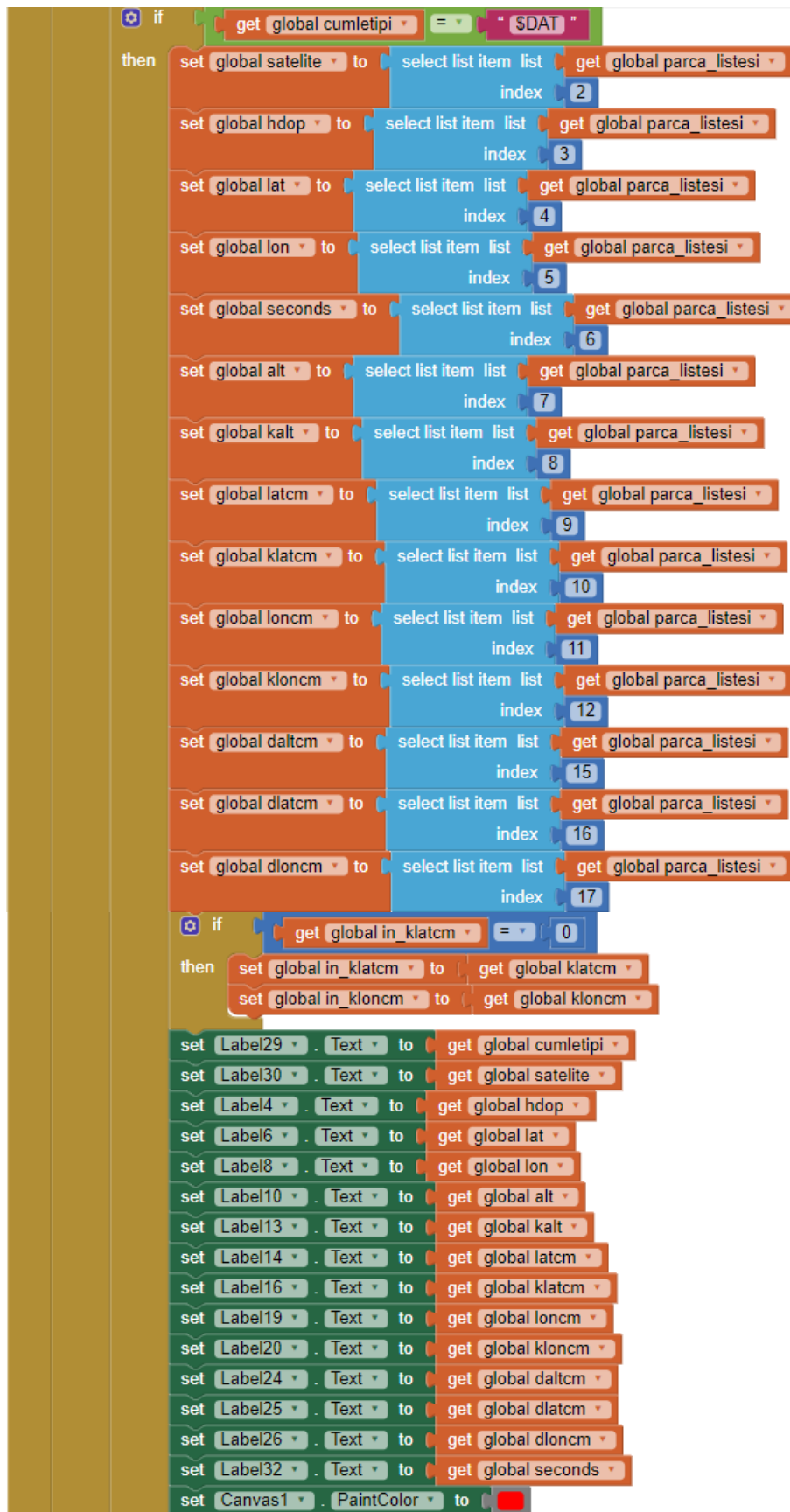
Fig. 4.12: Parsing the String and Assigning Them into Text Labels in App Inventor.
