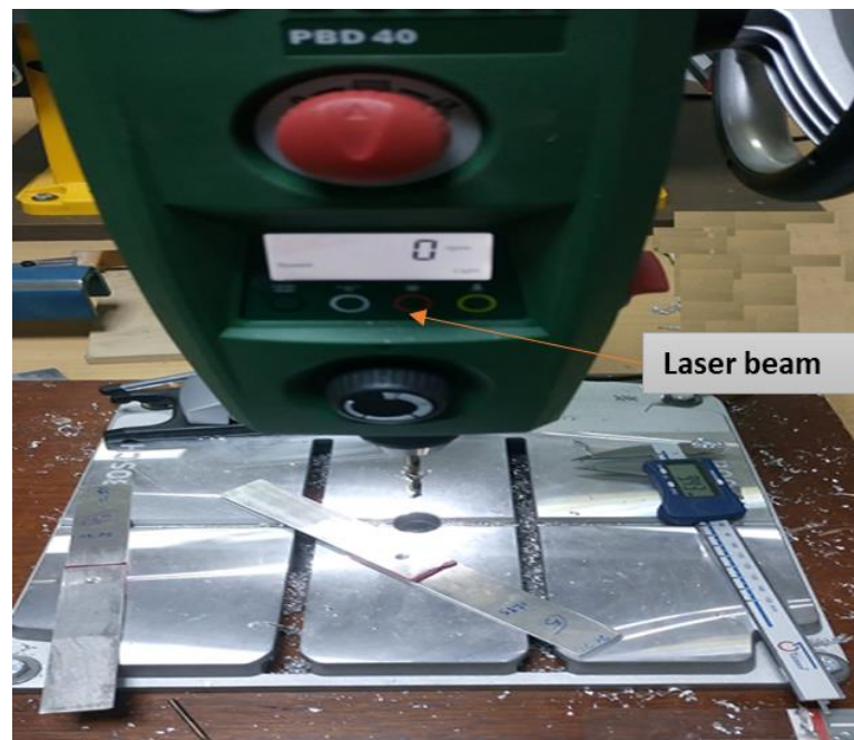
Figure 3.6: Drilling machine with laser alignment.
