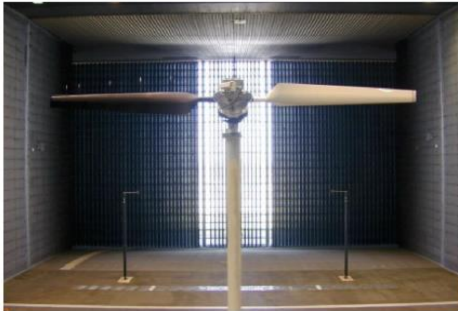
Figure 4.1. NREL-VI Wind Turbine Inside the NASA Ames Wind Tunnel. [77]
