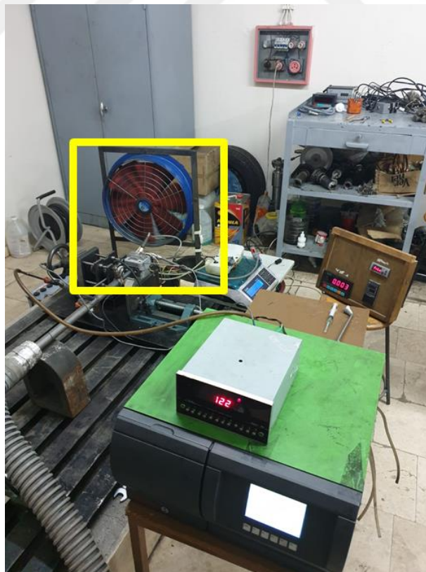
Figure 5.16: External cooling fan
