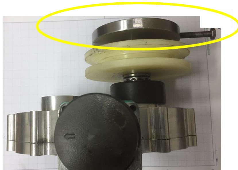
Figure 5.4: Initiator for magnetic pickup sensor and engine speed measurement sensor.
