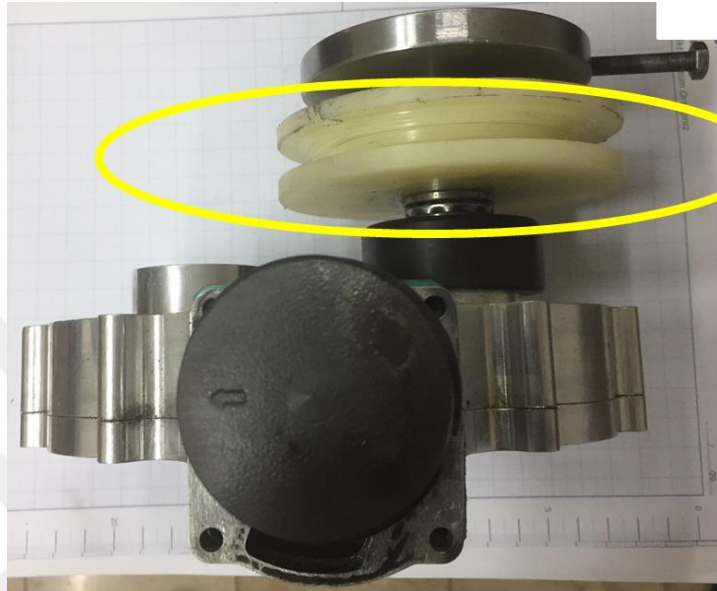
Figure 5.2: Pull start pulley and thrust ball bearing on the output shaft.
