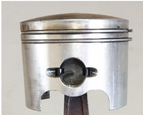
Figure 4.38: Piston, piston pin, and piston rings
