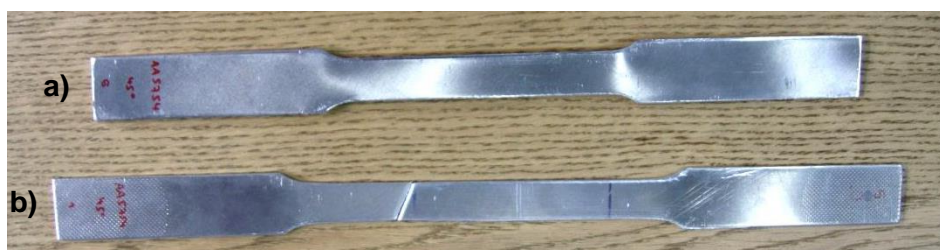
Figure 4.4: AA5754-H22 45° tensile test specimen: a) before the tensile test b) after the tensile test
