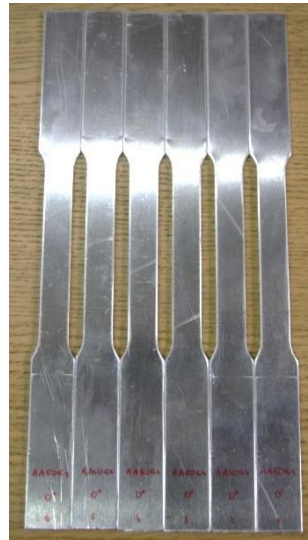
Figure 4.2: Set of tensile test specimens (AA6061-T6, 0°)
