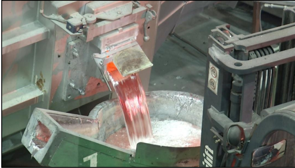
Figure 3.2: Transferring the liquid metal from melting furnace to transfer ladle [NN15]
