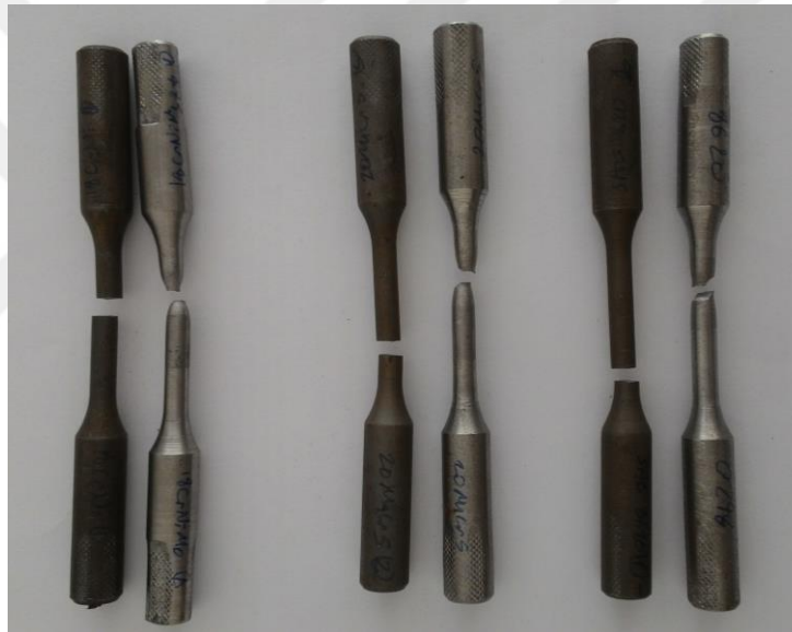
Figure 6.14 Tensile specimens, left to right 18CrNiMo7-6, 20MnCr5, 20NiCrMo2-2
