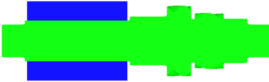
Figure 4.9 Interference fit layshaft model with gear hub
