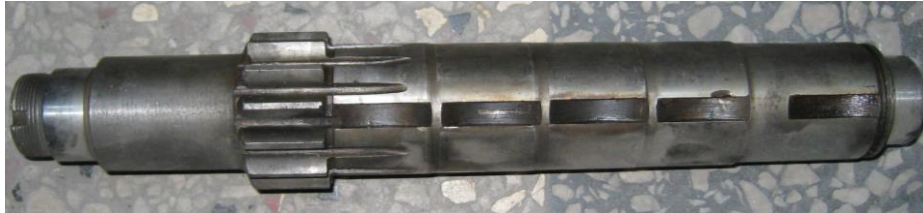
Figure 4.1 Keyway slotted layshaft, the manufacturer is unknown
