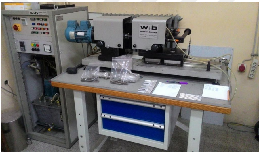
Figure 6.16 RB Fatigue test bench Walter+Bai AG UBM 5-200 Nm
