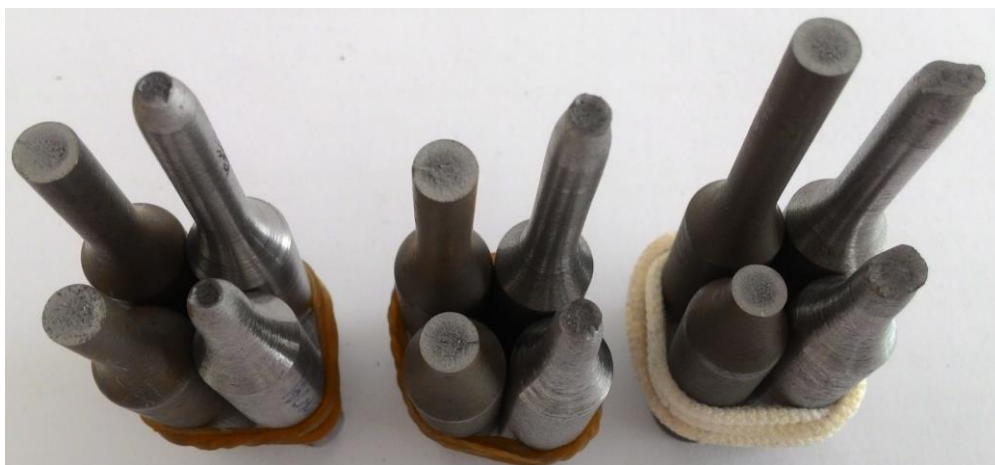
Figure 6.15 Fracture surface left to right 18CrNiMo7-6, 20MnCr5, 20NiCrMo2-2
