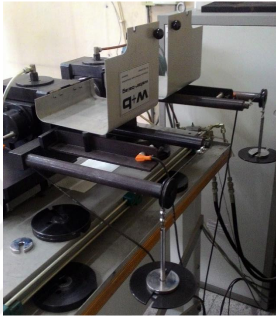
Figure 6.18 Interchangeable weights to create constant bending stress
