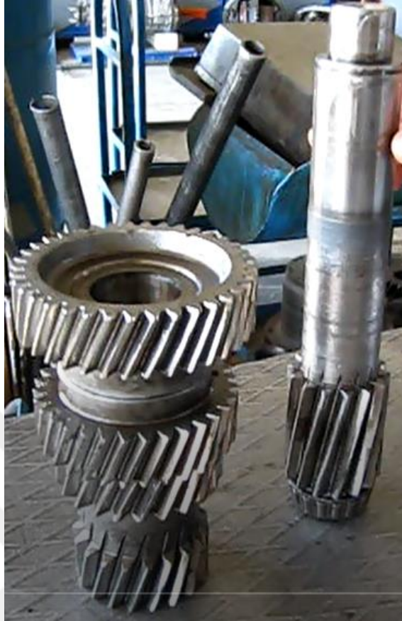
Figure 4.3 Interference fitted gears and flat surface layshaft (ZF)
