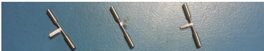
Figure 6.6 Manufactured tensile test specimens
