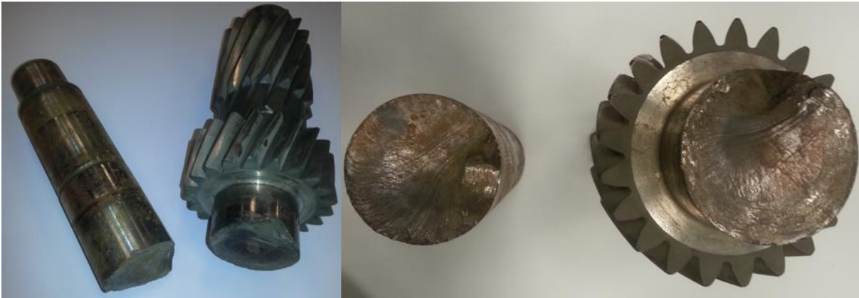
Figure 2.10 Failure of a construction truck transmission layshaft
