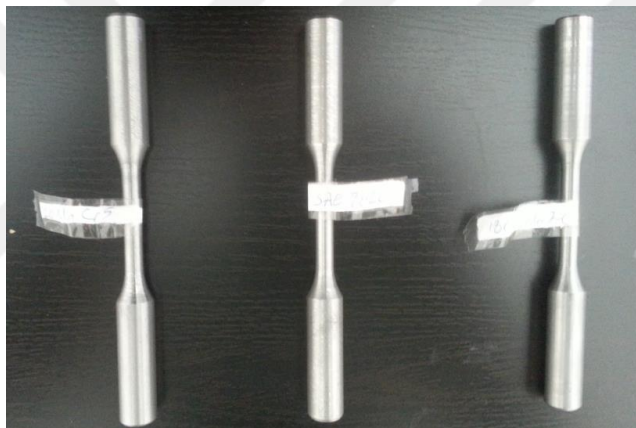
Figure 6.21 Specimens for each material group before heat treatment
