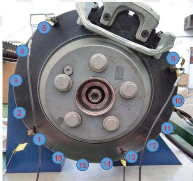
Figure 3.12: The experimental setup for the brake assembly and the measurement points.
