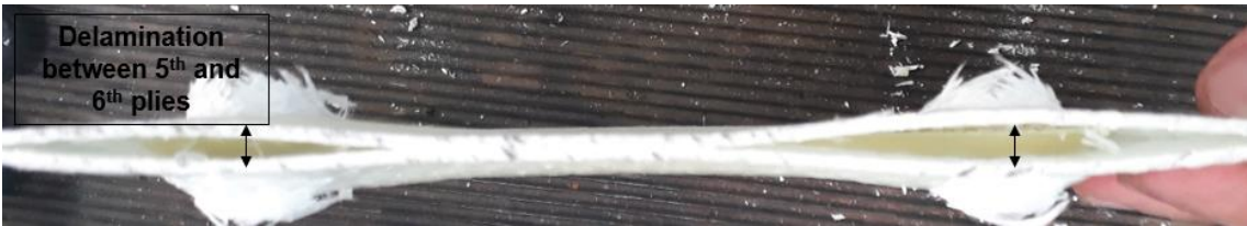
Figure 5.17. Delamination at polymer inserted specimens
