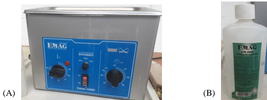
Figure 4.7. (A) Ultrasonic Vibration Machine and (B) Cleaning Agent.
