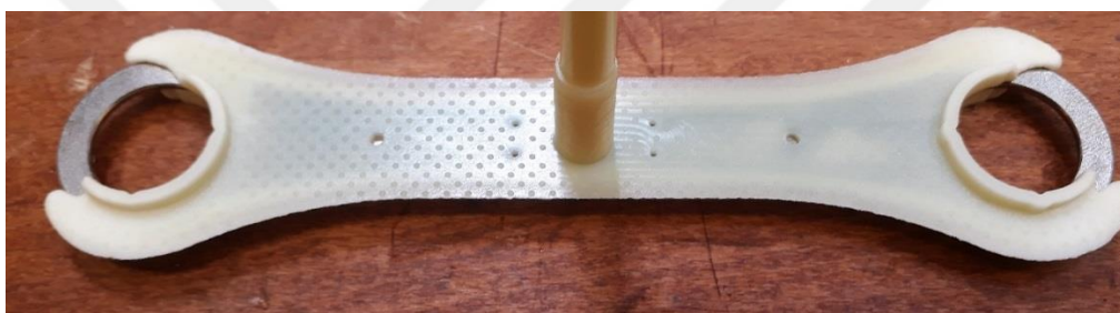
Figure 4.12. Poor filling of the cavity at injection molding process
