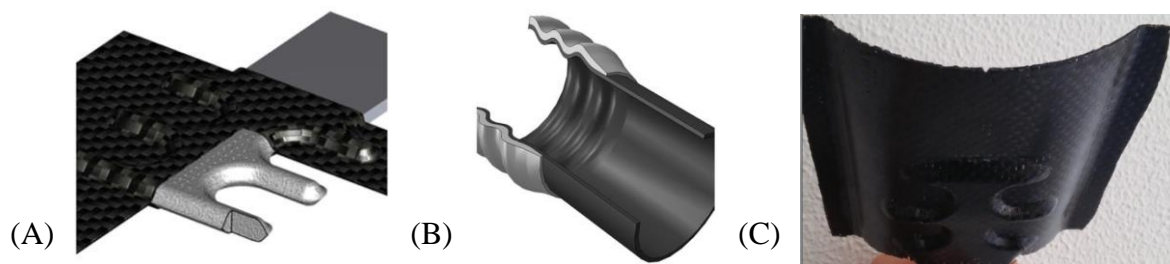
Figure 2.13. Customized contact zones: (A) Inclined contact zone and (B) curved contact zone and, (C) curved and inclined contact zones combined. (A) and (B) retrieved from (Kießling et al. 2016, p.4).
