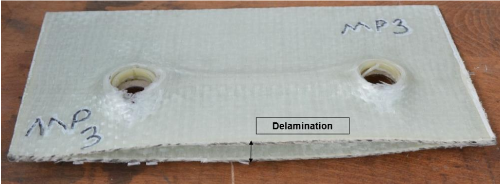
Figure 5.20. Delamination failure at specimen MP3
