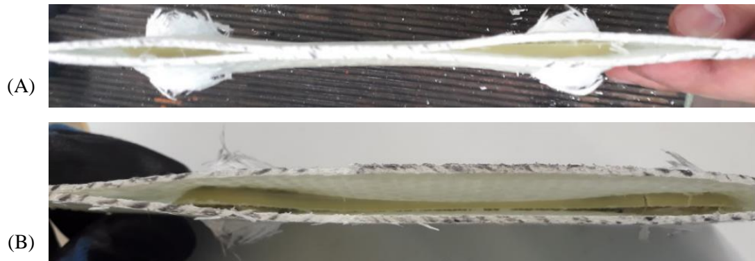
Figure 5.27. Delamination at (A) polymer inserted specimen and (B) metal-polymer inserted specimen
