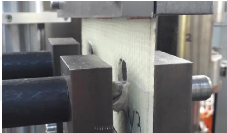
Figure 5.6. The crush of the composite around the hole as the pin moves through*
