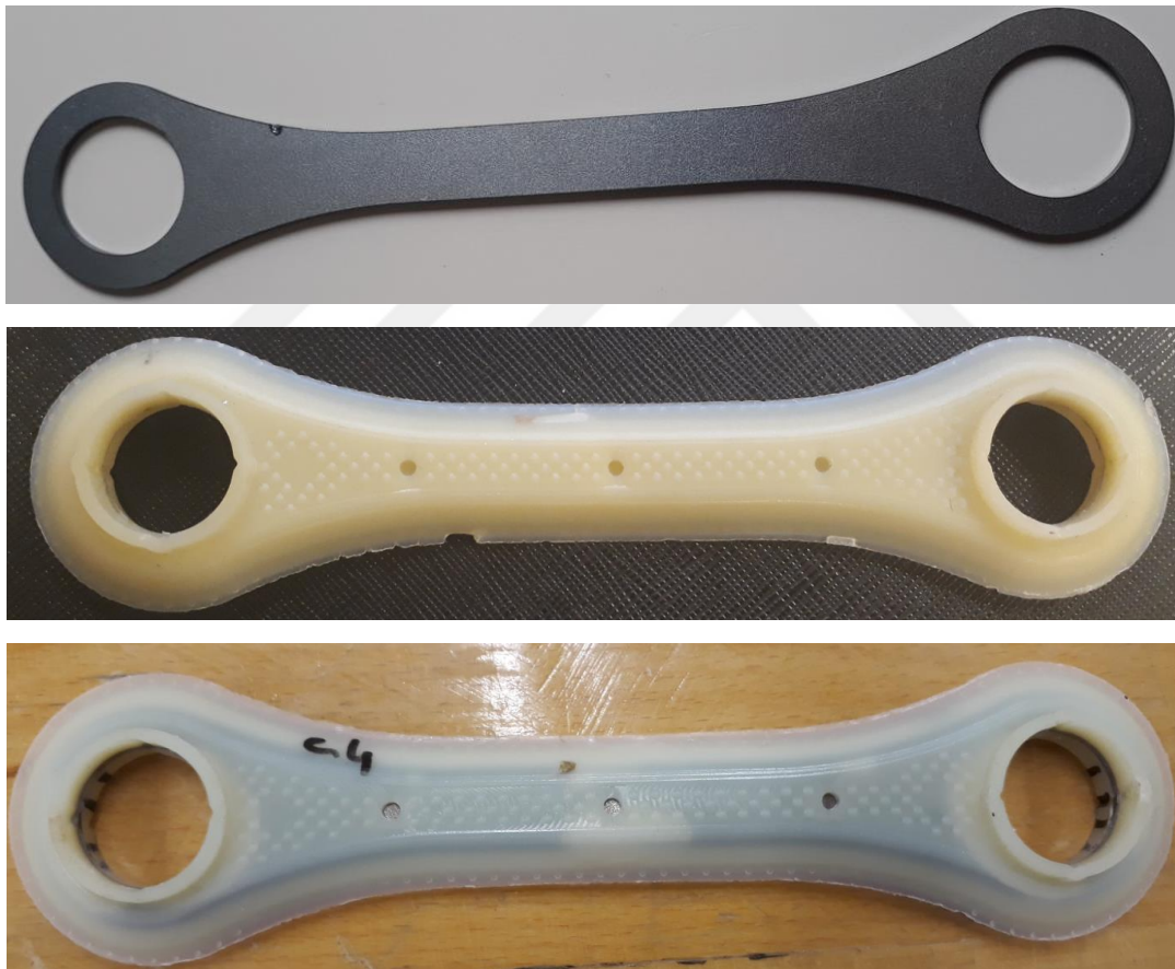
Figure 4.1. Pictures of produced inserts. (Top) Metal insert, (middle) polymer insert, (Bottom) Metal-polymer hybrid material insert
