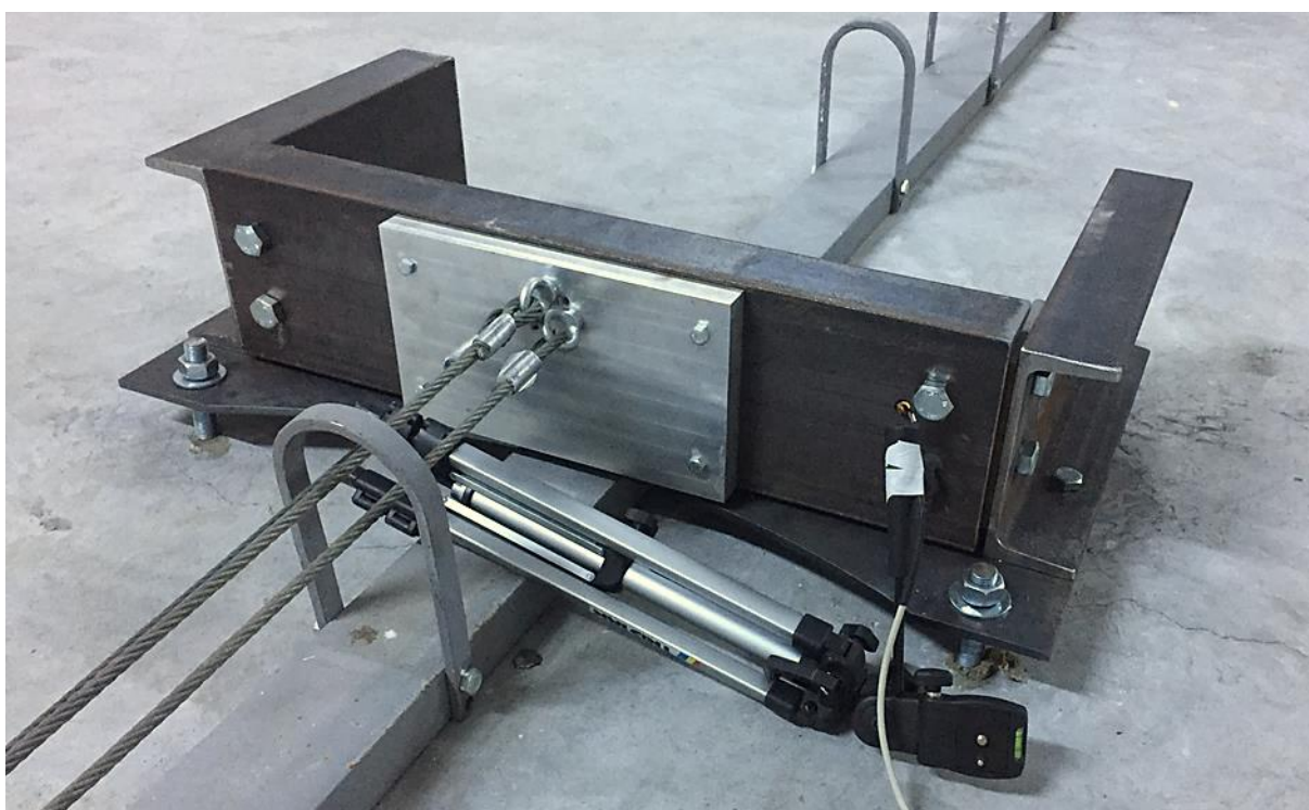
Figure 7.15: “Tower – Crane section” component attached to the test platform
