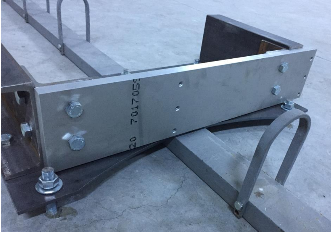
Figure 7.13: View of the flying sheave holder after test
