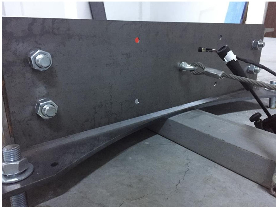
Figure 7.4: Closer view of steel rope attachment and temperature sensor
