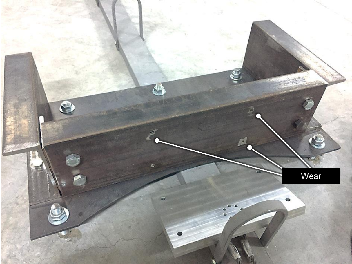
Figure 7.16: Tower crane section part after the test
