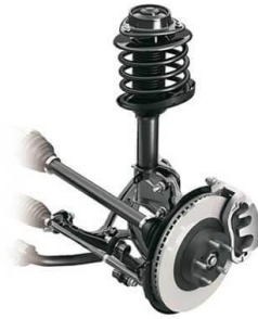
Figure 2.24: A suspension system with a coil spring [33]
