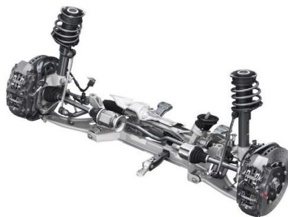
Figure 2.37: Audi TTRS with MacPherson strut type suspension [49]
