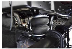
Figure 2.31: Air suspension system example [44]
