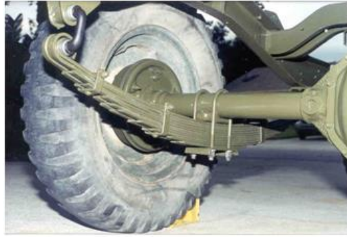
Figure 2.21: Leaf springs used for suspension in a heavy vehicle [31]
