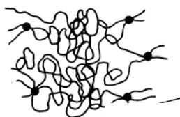
Figure 2.7: Molecular structure of an elastomer [10]
