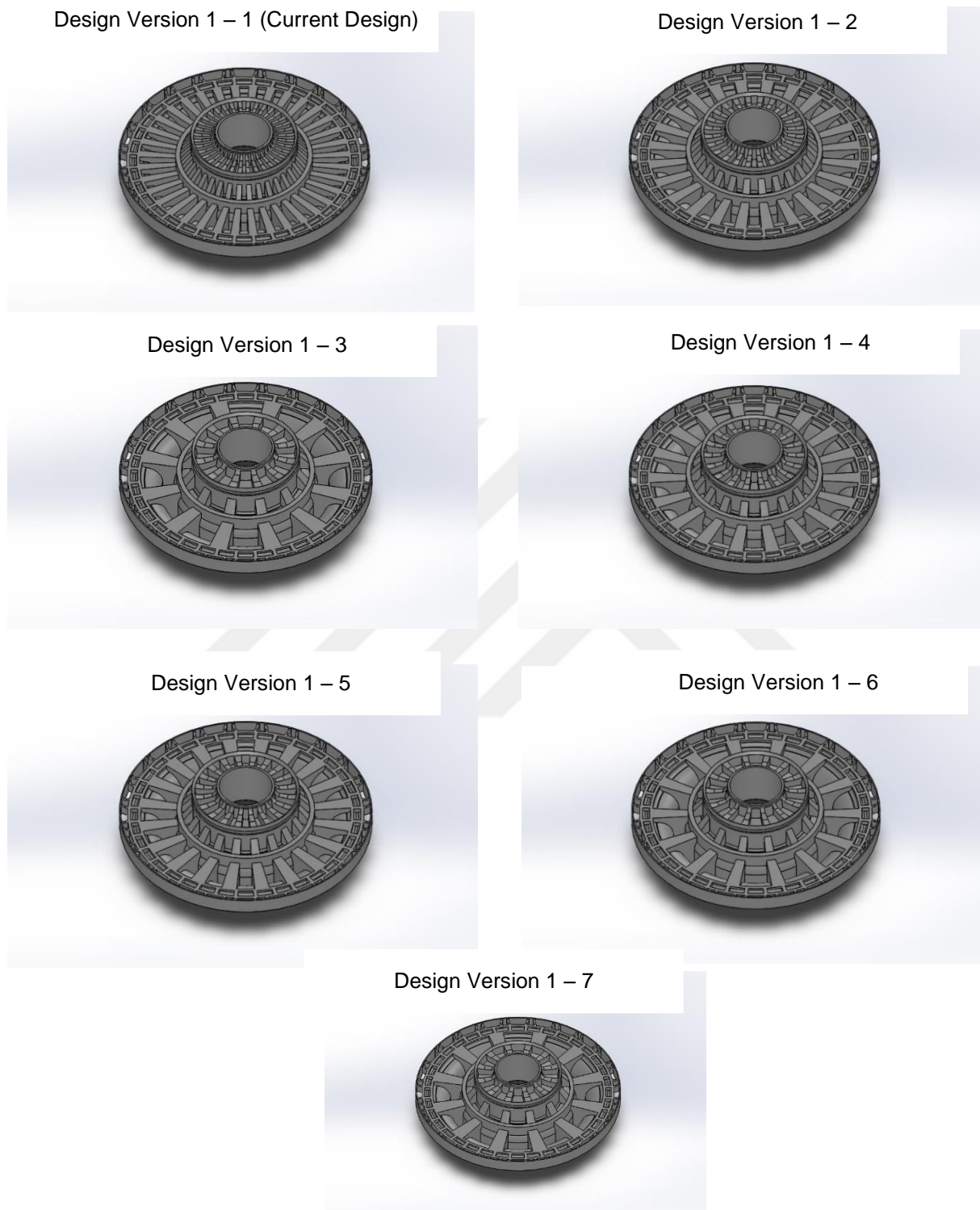
Figure 3.7: Modified upper spring seat designs – Design Version 1
