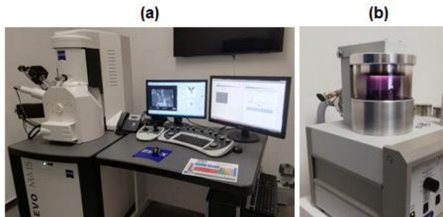
Figure 4.26: (a) Scanning electron microscope (SEM) and (b) Gold plating process prior to SEM
