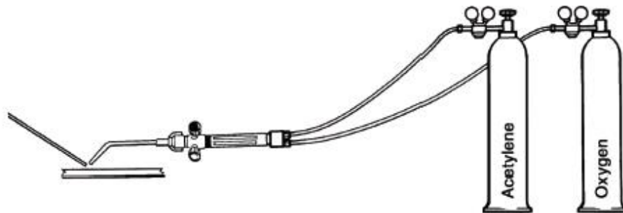
Figure 2.4: A gas welding set [Wem03]
