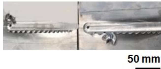
Figure 3.7: Excess flash formation
