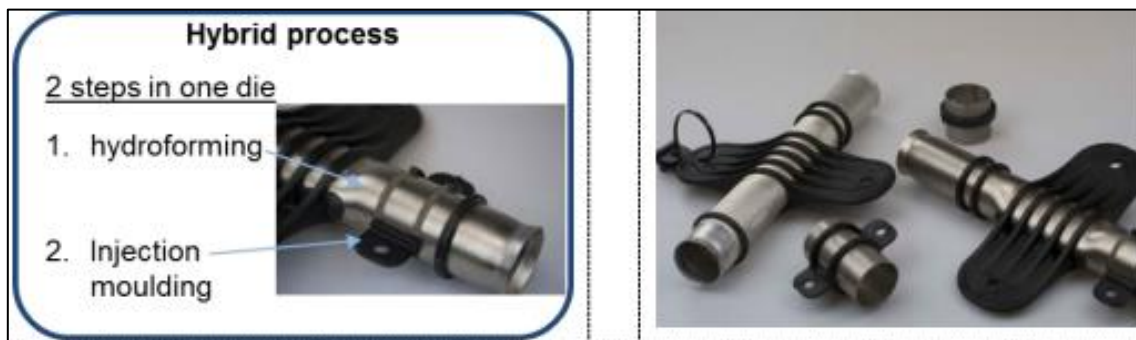
Figure 2.17 Process combination of hydroforming and injection moulding (Drossel et al., 2016)
