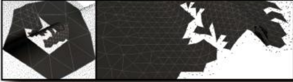
Figure 4.1 : Left: Surface constructed using only local curvature. Right: Surface constructed using a guidance field. Figure taken from [34].
