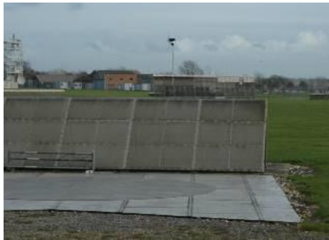
Figure 6.1 : Fences used to reduce interference from reflections (Hopwood, 2011).
