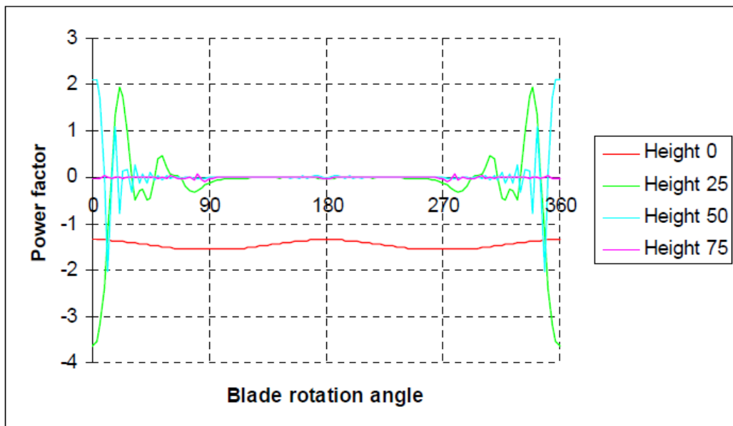
Figure 5.5 : Time variation of power behind rotating 50x3 m turbine blade (18 km to transmitter, 1 km to target; radar frequency 3 GHz).
