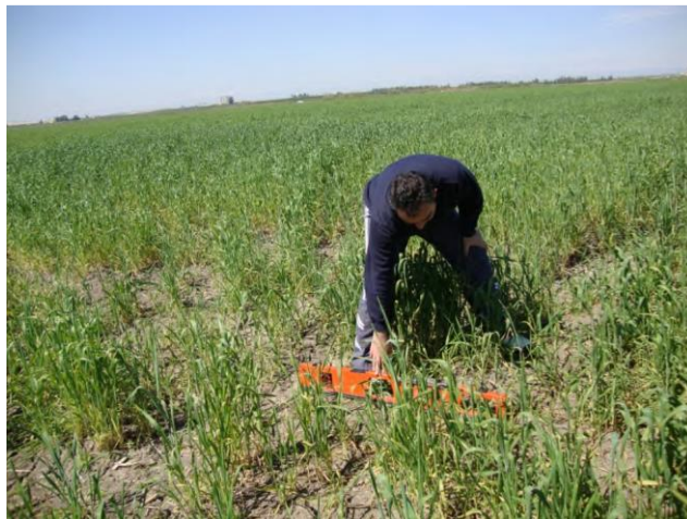
Figure 6.3 : A field photo showing EC measurements by EM-38 device.
