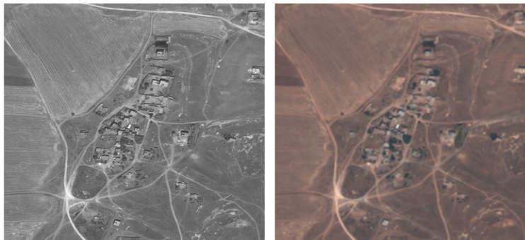
Figure 5.13 : Original Pleiades panchromatic image (left) and VDSR result of multispectral Pleiades image (right) by a scale factor of 4.
