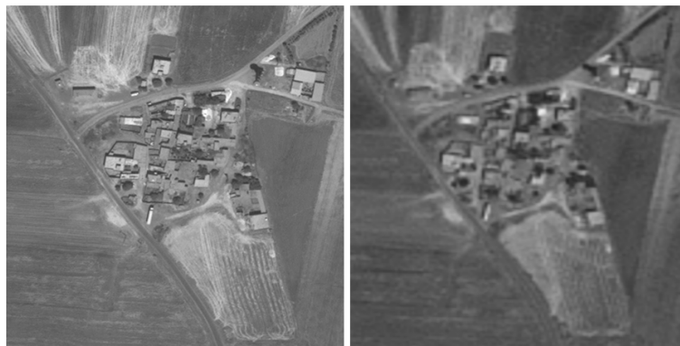
Figure 5.14 : Original Pleiades panchromatic image (left) and VDSR result of multispectral Pleiades image (right) by a scale factor of 3.
