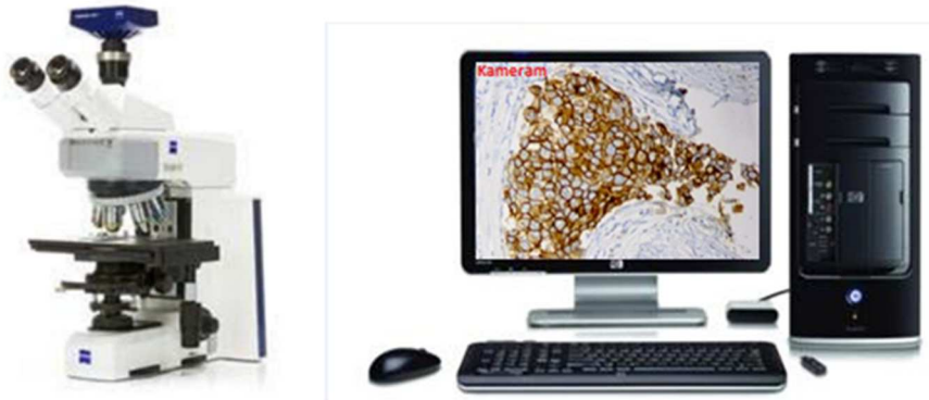
Figure 2.1 : Image acquisition system. Microscope: Zeiss Axio Scope A1, Camera: Argenit Kameram 2 CCD, Software: Argenit Kameram: Computer: Intel i7 processor, 8 GB RAM, 1TB HDD, Win7 Professional OS.
