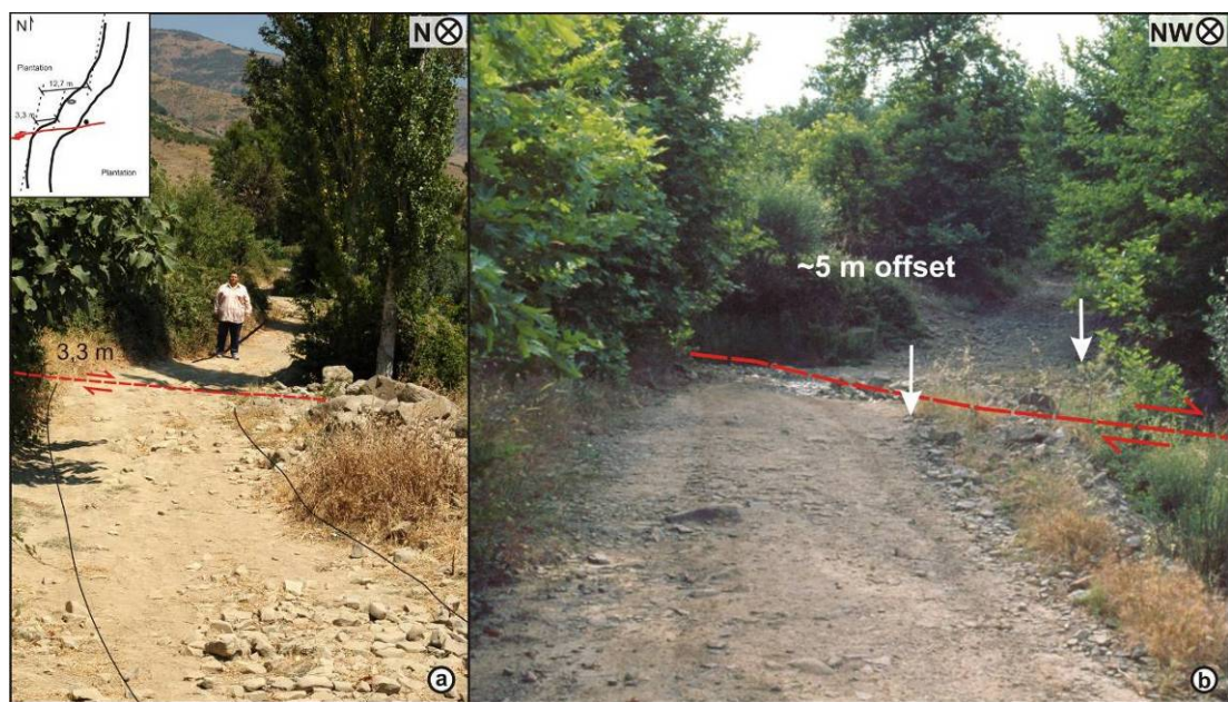
Figure 5.7 : Two road offset near Gaziköy. Location of a) is given in Figure 5.5. The road appears to be an ancient pavement. We measured 3.3 m of right-lateral co-seismic and 12.7 m cumulative displacement on this road. The inset illustrates the offset in map view. b) Another offset road (~ 5 m) located ~1 km to the west.
