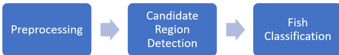
Figure 2.2 : Scheme of the proposed fish detection method.
