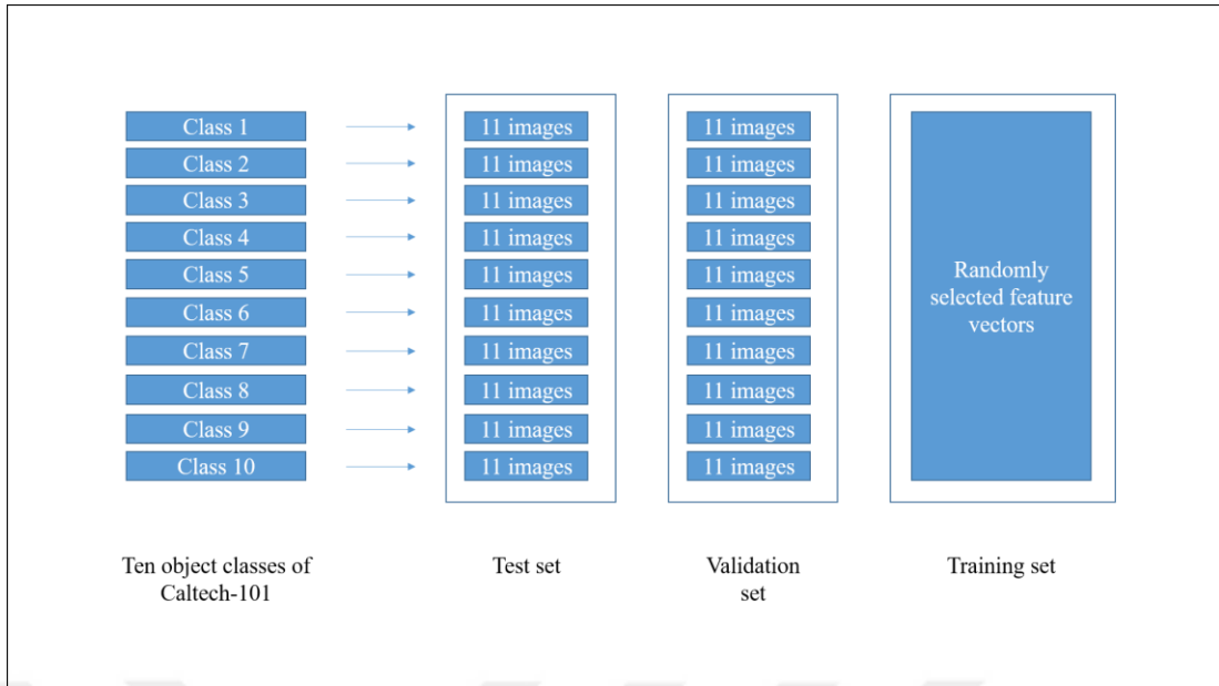
Figure 4.6 : Design of the test, training and validation sets of the dimensionality reduction algorithm. The test set of the system is used for object recognition tests. The validation set has the same amount of images with the test set and is used to validate the system. The training set of the system consists of randomly chosen vectors which are twice the size of vectors in test set.
