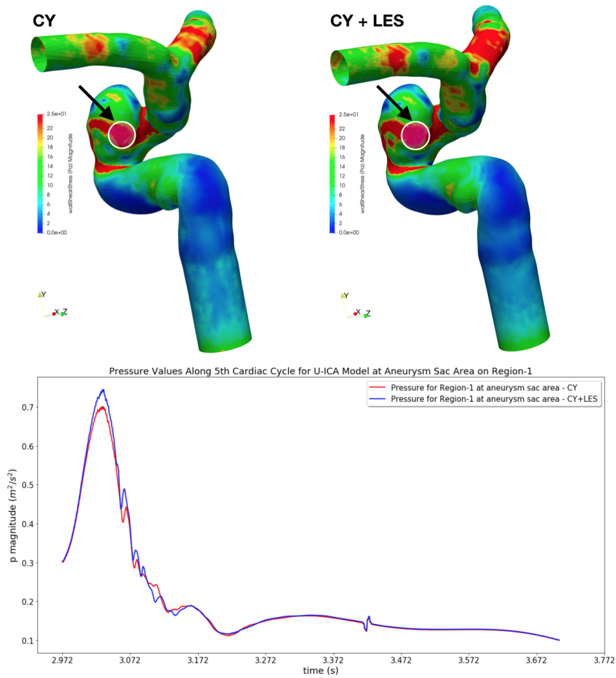
Figure 5.13 : Pressure behavior has been observed during last cardiac cycle within U – ICA geometry for the region-1 on the aneurysm sac area which is indicated with white circle. CY indicates Carreau-Yasuda viscosity model and LES indicates Large Eddy Simulation.
